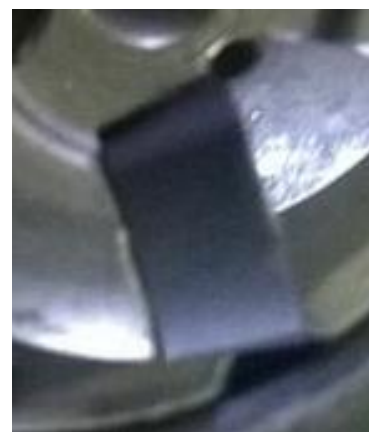
wear insert after 240 minutes of work
